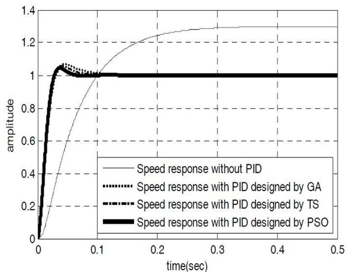
**Fig 9 : System responses of BLDC with PID controller designed by GA, TS and PSO**
