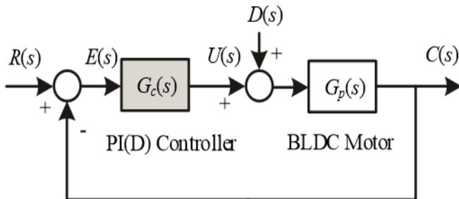
Fig 4 : PI(D) control loop
