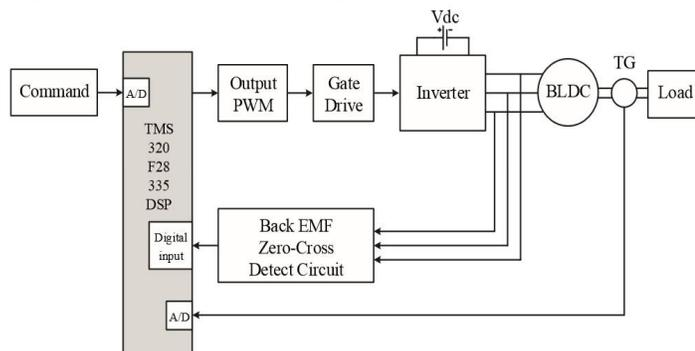
Fig 3 : DSP based speed control of BLDC motor
