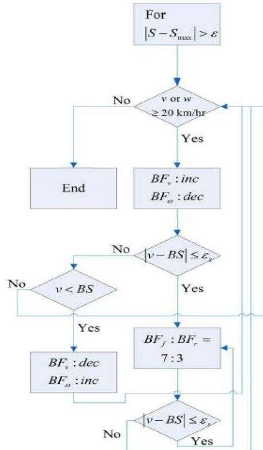
Fig 7 : Flow chart of the adjustment for the brake forces.
