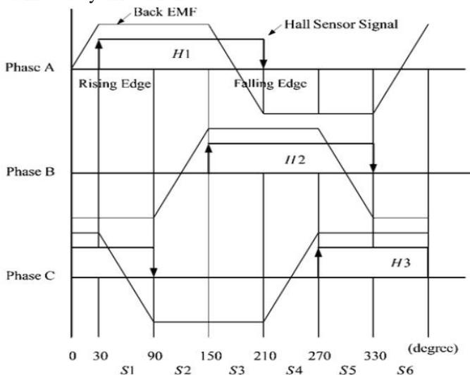
Fig 1 : Back EMF and Hall effect sensor signals
