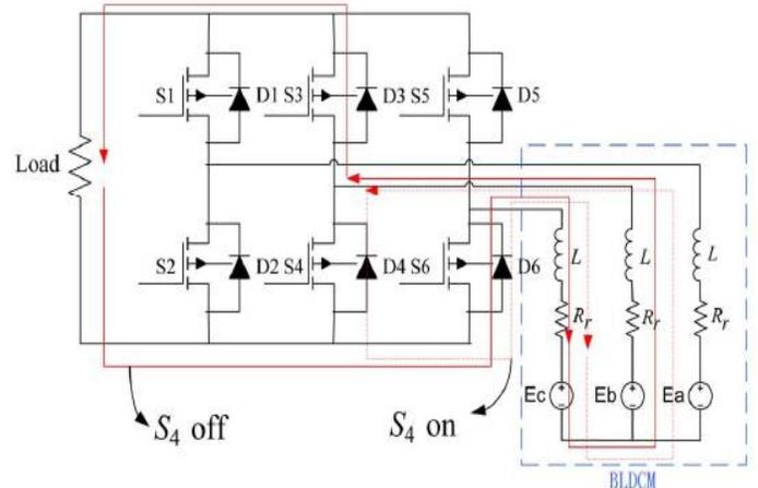
Fig 6 : Current conduction loop in short-circuit and kinetic brakemode, which correspond to S4 on and S4 off, respectively.
