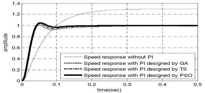
**Fig 8 : System responses of BLDC with PI controller designed by GA, TS and PSO**
